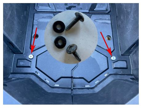
Step 3. Install the mount utilizing the (2) flange head bolts with a 10mm socket and ratchet. The mount is reversible so that the toolboxes or cooler can be inserted and opened left or right handed.
