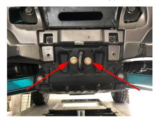
Step 3: Cut off the plastic area where you removed the Torx screws.
