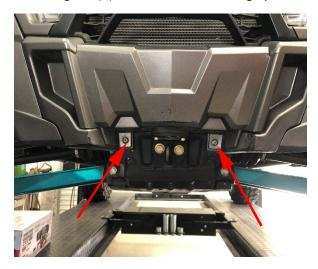
Step 2: Remove the factory tow hook by removing the (2) 15mm bolts. Leave the backing plate in place.
