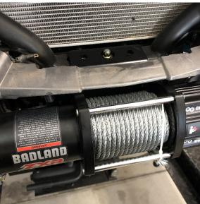
Step 6: Remove the winch mounting plate. Install the winch on the mounting plate with the hardware that comes with your winch.
