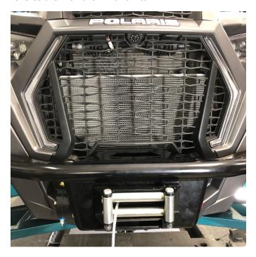
Note: Some fairleads may need to have the holes enlarged or moved to bolt onto the bumper. The badlands roller fairlead shown needed to have the holes slotted ½ the diameter of the existing holes.
