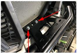
Step 11: Install the remaining (2) M8 bolts and nylock nuts through the bottom two holes. Then tighten all hardware previously installed.
