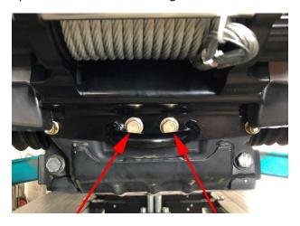
Step 8: Insert (2) M8 bolts with nylock nuts in the outside holes. You may need to clearance your plastic more depending on how much you cut off in Step 3. Snug the bolts and nuts.
