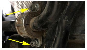
Step 6: Slide the sway bar support bracket over sway bar and into position.
