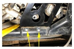
Step 9: Gently raise the motor with the pry bar and install the motor mount bolt. Tighten the bolt to the factory spec with the 15 mm socket.
