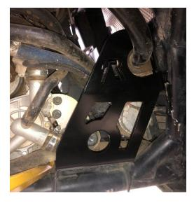
Step 7: Reinstall the carriage bolts and nuts on the sway bar mount to help hold the bracket in position. DO NOT TIGHTEN.
