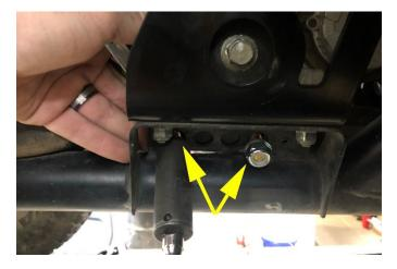
Step 14: Move the sway bar into position with the sway bar links and install the factory bolt and nut on BOTH sides. Tighten to the factory spec with the 15 mm wrench and 15 mm socket.
