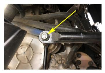
Step 2: Remove the nuts from the bottom motor mount bolts on BOTH sides with the 13 mm socket.
