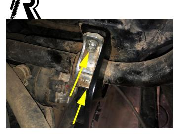
Step 12: Install the 2 nuts on the bottom motor mount bolts on both sides. Tighten to the factory spec with the 13 mm socket.
