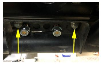
Step 13: Tighten the 2 new M10 bolts and nuts using the 15 mm wrench and 17 mm socket on both sides.
