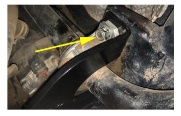
Step 8: Install the 2 provided M10 bolts through the back side of the frame and sway bar support bracket. It helps to gently raise the motor with the pry bar on the passenger side to clear the hose. Install the 2 washers and nylock nuts. DO NOT TIGHTEN.
