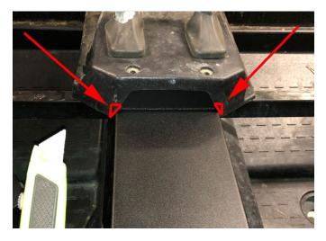
Step 6: Once the corners are trimmed enough to fit all the way down you can lift the rear console delete plate and install the cigarette lighter wires. Then put the plate back into position and reinstall the fasteners in the factory positions.
