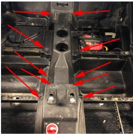
Step 3: Remove the rear center console by lifting the rear up first. You can lift the rear portion of the front console to make it easier. Remember to unhook the cigarette lighter wires. If you have rear harness' that are bolted in you will need to remove the bolts with a M16 and M19 wrenches or sockets. If you have 3 point seat belts the rear center console can slide over them.
