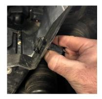
starting with the leading end. Also lift up on the rear portion of the front console. You will need to trim two small triangles of plastic from the front console for it to go all the way down.
