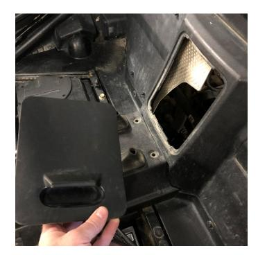
Step 8: Install the rear block off plate by sliding it horizontal from the front then rotating the front bottom edge down. You can reach through the access hole to hold the plate in position while you install the two factory plastic clips. Then reinstall the rear access panel.
