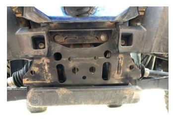
Step 2: Insert the (4) M10 bolts from the outside through the tow hook and frame. Put the (4) washers and nylock nuts on the back side of the frame. Tighten the hardware.
