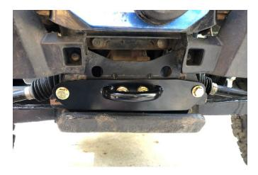
Step 3: Here you can see where the plastic normally is indicated by the green lines. The red line indicates the area that you may need to trim with a razor blade for the plastic fascia to clear the bolt heads. The plastic indicated by the green lines was completely removed to better show the tow hook and is not necessary for the installation. Reinstall the front fascia if removed.
