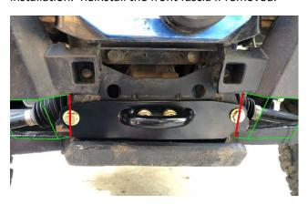
Step 4 (Optional): If you are using the tow hook as a tie down point and use straps with large hooks, you may need to change the center two bolts. You can use (2) 3/8-16 x 1" grade 8 bolts with washers. It should provide just enough clearance.
