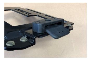
Step 7: Attach the front part of the seat base to the main part of the seat base with the supplied (4) carriage bolts and nylock nuts. Insert the carriage bolts from the inside into the square hole so they point outward. The bottom set of holes are for the 3.5° setting, the middle holes are for the 5.2° setting, and the top holes are for the 7° setting.
