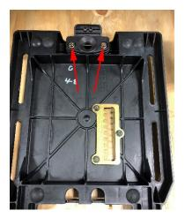
Step 4: Insert the (6) factory rubber bumpers into the (6)  $\frac{1}{2}$  holes in the new seat base.
