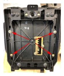
Step 2: Remove the (6) rubber bumpers/isolators from the stock seat base.
