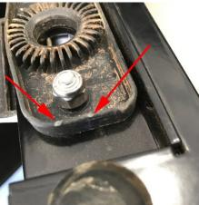
Step 9: Attach the new seat base to the seat with the (4) factory torx bolts removed in step 1. Reinstall the seat and get to riding!
